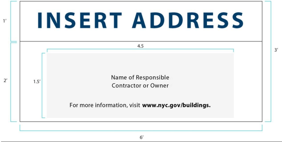
Figure 4: Sidewalk Shed Parapet Panel Layout
